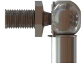
401 000 013 Ball Joint Material Information; Steel Sheet + 11SMnPb30 Surface Treatment; White Zinc Plated General Tolerances; DIN ISO 2768-medium
